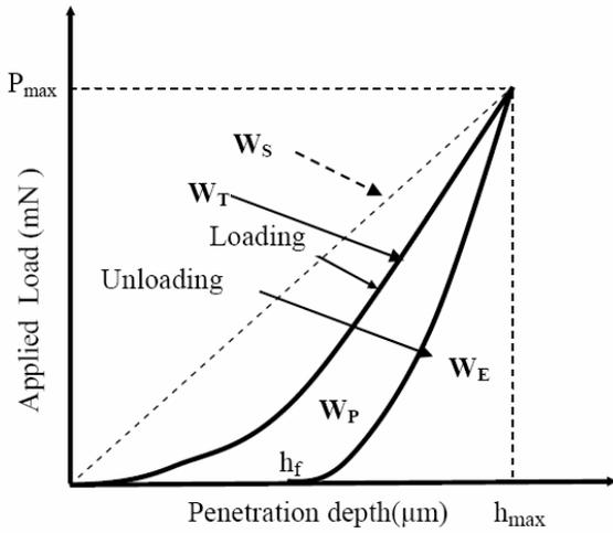
Fig. 1. Typical indentation cycle showing load-unload curves.
