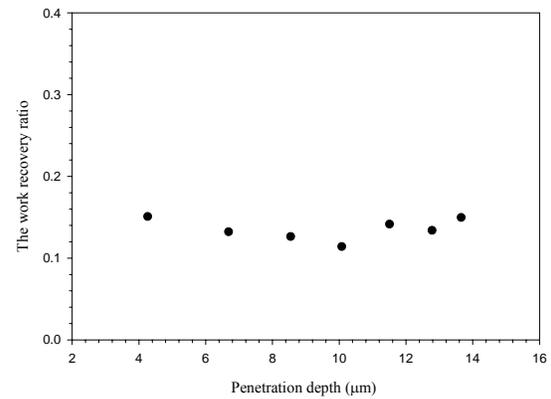
Fig. 4. Relationship between the work recovery ratio and penetration depth for BSCCO sample.
