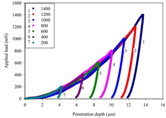
Fig. 2. Load-penetration depth behavior of BSCCO sample.
