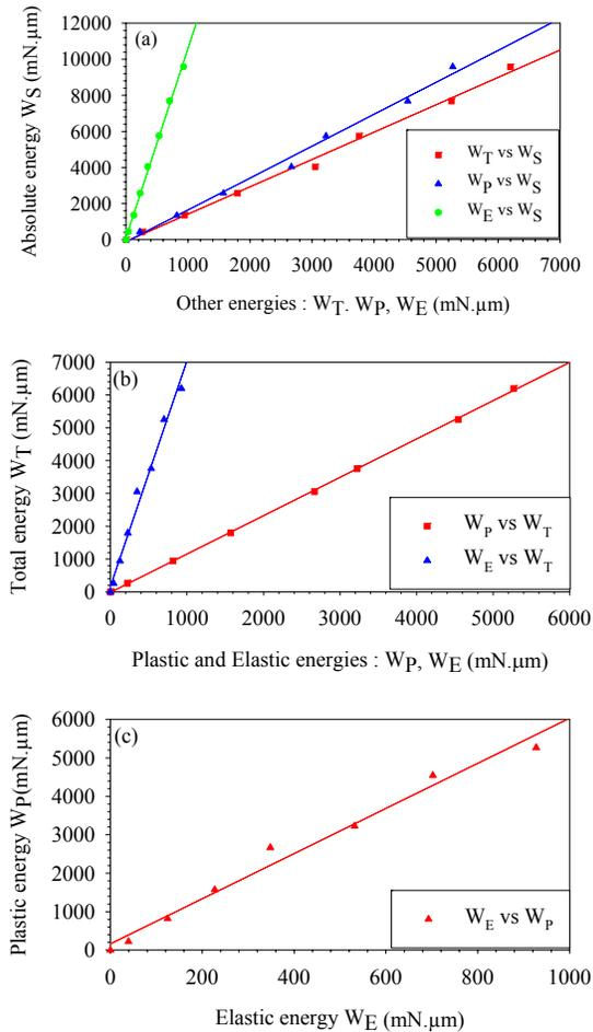
Fig. 3. Correlation between energetic quantities involved in BSCCO indentation with Vickers tip (a) Variation of absolute energy ( $W_S$ ) versus the other energies. (b) Variation of total energy ( $W_T$ ) versus elastic and plastic energies. (c) Variation of plastic energy ( $W_P$ ) versus elastic energy ( $W_E$ ).
