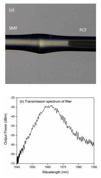
Fig. 2. All-fiber bitaper MZI. (a) Image of the fiber taper; (b) Transmitted light source profile of the MZI
