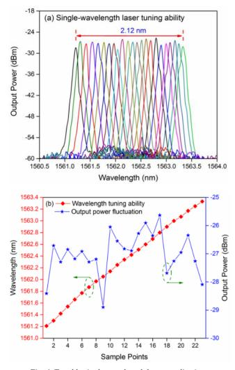
Fig. 4. Tunable single-wavelength lasers realization.
