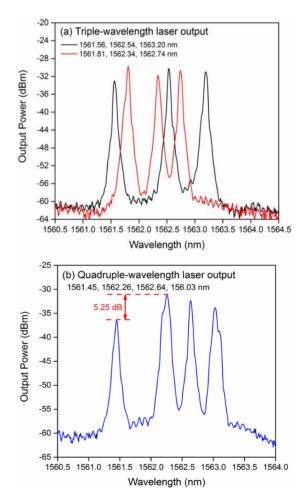
Fig. 6. Tunable triple- and quadruple-wavelength tuning output. (a) Triple-wavelength output;
