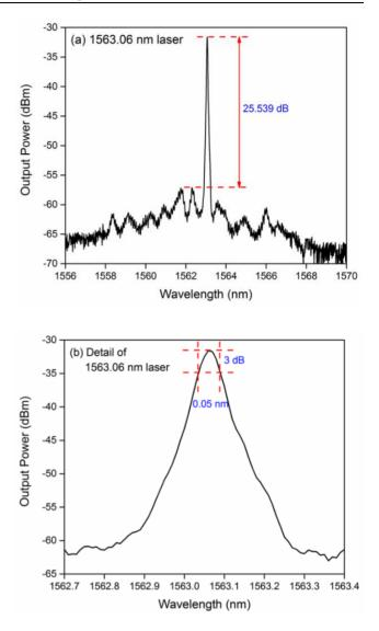
Fig. 3. Laser output of 1563.06 nm. (a) Spectrum ranging from 1556 to 1570 nm; (b) Spectrum ranging from 1562.7 to 1563.4 nm
