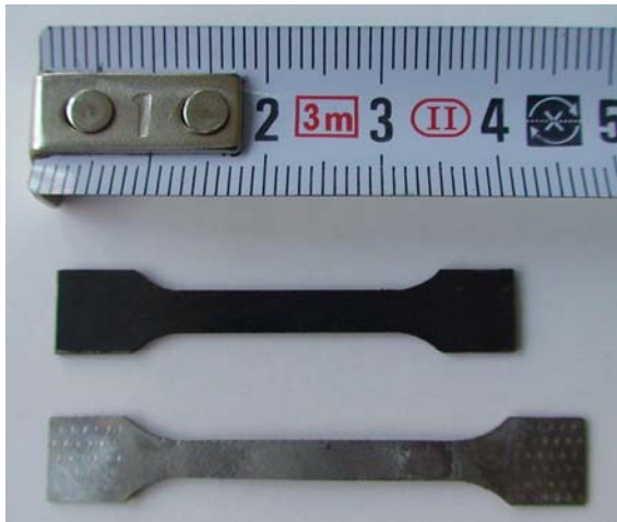
Fig. 2. Tensile specimens after spark erosion cutting (dark) and after 10 constrained recovery cycles, grinding polishing and etching.
