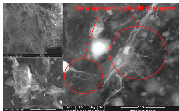
Fig. 9. SEM images with fiber-like morphology of LGGNi complexes obtained in presence of SiNW.
