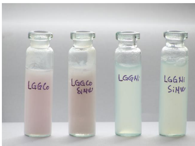
Fig. 1. Appearances indicating the metal complex formation in presence (absence) of SiNW particles (homogenous dispersions and gel-like for LGGNi/SiNW).
