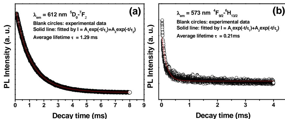
Fig. 5. Decay curves of the CaWO<sub>4</sub>:Eu<sup>3+</sup> (a) and CaWO<sub>4</sub>:Dy<sup>3+</sup> (b) phosphors.
