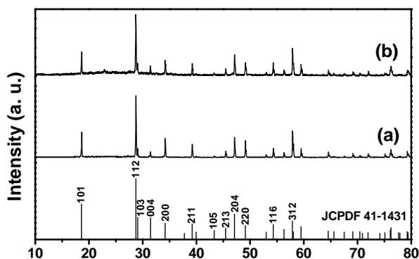
Fig. 1. XRD patterns of pure  $\text{CaWO}_4:\text{Eu}^{3+}$  (a),  $\text{CaWO}_4:\text{Dy}^{3+}$  (b), and the standard data for  $\text{CaWO}_4$  (JCPDS 41-1431).
