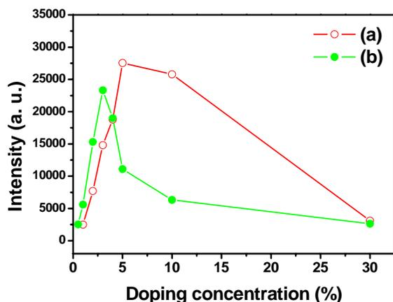
Fig. 6. The PL emission intensity of Eu<sup>3+</sup> in CaWO<sub>4</sub>:Eu<sup>3+</sup> (a) and Dy<sup>3+</sup> in CaWO<sub>4</sub>:Dy<sup>3+</sup> (b) as a function of the doping concentration.
