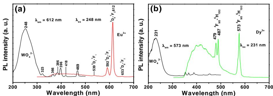
Fig. 4. Excitation (left) and emission (right) spectra of the  $\text{CaWO}_4:\text{Eu}^{3+}$  (a) and  $\text{CaWO}_4:\text{Dy}^{3+}$  (b) phosphors.
