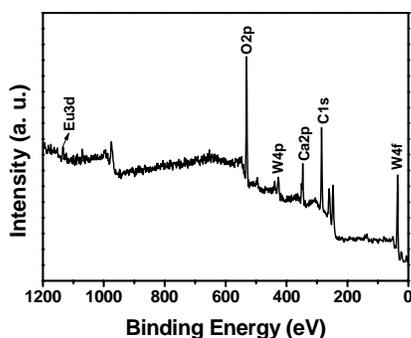
Fig. 3. XPS of the as-synthesized  $\text{CaWO}_4:\text{Eu}^{3+}$ .
