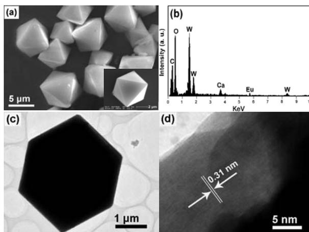
Fig. 2. SEM image (a), EDS (b), TEM image (c), and HRTEM image (d) of the as-synthesized  $\text{CaWO}_4:\text{Eu}^{3+}$ .
