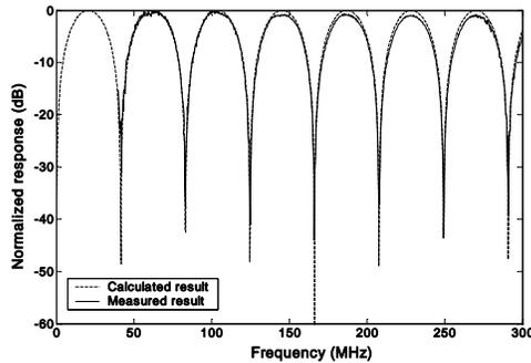
Fig. 2. Measured and calculated response of the bandpass filter without tuning the time delay line
