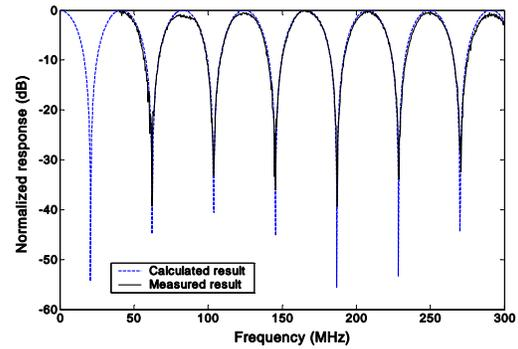
Fig. 4. Measured and calculated response of the low pass filter without tuning the time delay line
