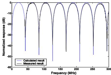
Fig. 3. Measured and calculated response of the bandpass filter when the time delay is tuned to 300 ps.
