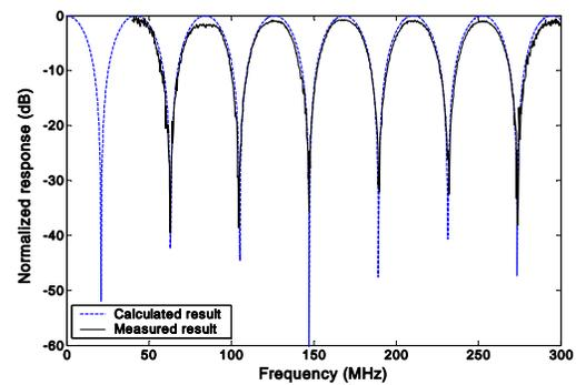
Fig. 5. Measured and calculated response of the low pass filter when the time delay is tuned to 300 ps.
