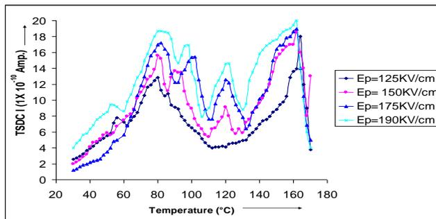
Fig. 6. TSD current spectra of 100 MeV Ag-ion irradiated PVDF (20  $\mu$ m) at polarization temperature  $T_p = 80^\circ\text{C}$  for different polarization fields,  $E_p$ .
