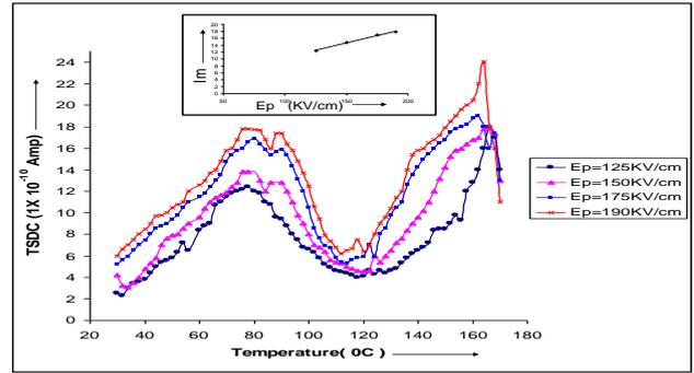
Fig. 4. TSD current spectra of Pristine PVDF (20  $\mu$ m) at polarization temperature  $T_p = 80^\circ\text{C}$  for different polarization fields, and Inset of the figure 4 shows the variation of peak current ( $I_m$ ) with  $E_p$  (kV/cm) for  $\beta$ -peak.
