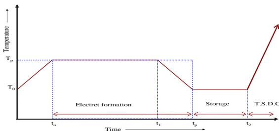
Fig. 2. Experimental schematic representation of TSDC procedure:  $T_0$ , initial temperature;  $T_p$ , polarization temperature;  $t_0$ , start of polarization;  $t_1$ , start of cooling;  $t_p$ , switching off the field  $E_p$ ;  $t_2$ , start of heating the sample and recording the current as the function of temperature.
