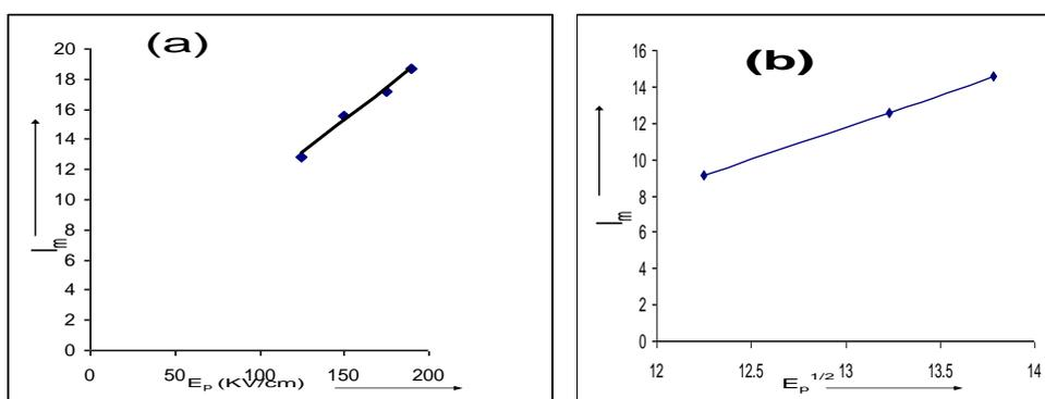
Fig. 7. Variation of peak current ( $I_m$ ) with (a)  $E_p$  (kV/cm) for  $\beta$ -peak (b)  $E_p^{1/2}$  for  $\alpha$ -peak in 100 MeV Ag-ion irradiated PVDF (20  $\mu$ m) samples at  $T_p = 80^\circ\text{C}$ .
