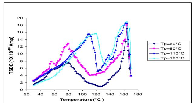
Fig. 5. TSD current spectra of 100 MeV Ag-ion irradiated 20 $\mu$ m PVDF thin film at polarization field  $E_p = 125$  kV/cm for different polarization temperature ( $T_p$ ).
