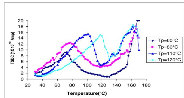
Fig. 3. TSD current spectra of  $20\ \mu\text{m}$  Pristine PVDF at polarization field  $E_p = 125\ \text{kV}/\text{cm}$  for different polarization temperature ( $T_p$ ).
