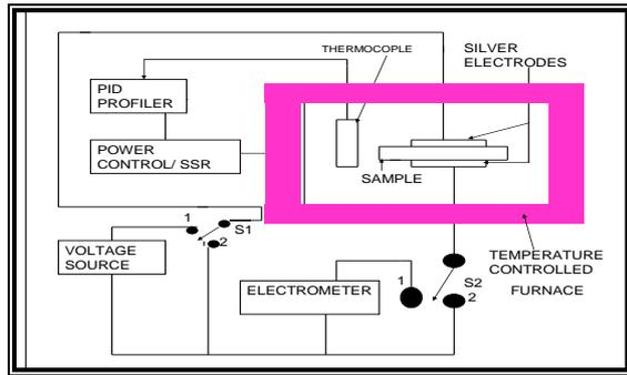
Fig. 1. Schematic diagram of the experimental setup for the TSDC measurements.
