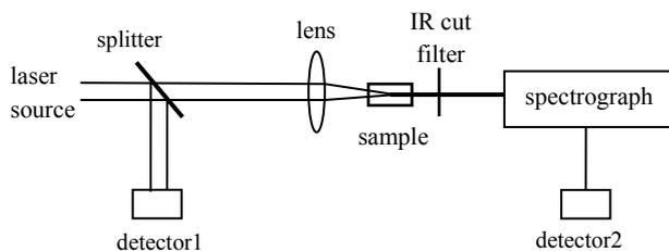
Fig. 1. The optical setup for three-photon photophysical measurements
