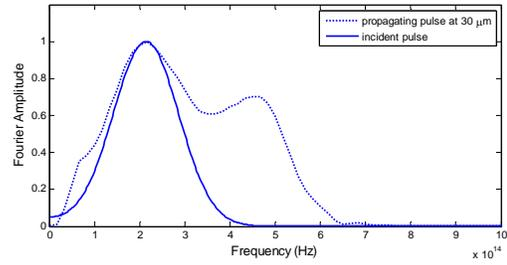
Fig.5: Frequency spectra of the incident pulse (solid curve), and the pulse which has propagated 34.2 μm in the nonlinear one-ring PCF.
