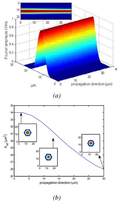
Fig.6: (a) Nonlinear mode profile in YZ plane at wavelength of 1.4 μm, with self-focusing effect along propagation direction, (b) The effective area evolution along the propagation path, with mode profiles in transverse plane (XY plane) at 3 μm, 15 μm and 30 μm in the propagation direction.
