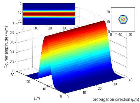
Fig.3: Propagating mode profile along the fiber axis for 37.5  $\mu\text{m}$  at wavelength of 1.4  $\mu\text{m}$ , top left plot is the YZ top view of the Fourier amplitude, top right plot is the linear mode profile at wavelength of 1.4  $\mu\text{m}$  which is the same along the propagation path.
