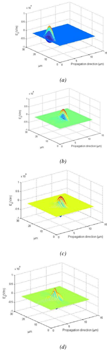
Fig.4: Propagating pulse (a) shows the pulse entering the problem space after 9 fs, (b) shows the pulse reaching the midpoint of the space after 38 fs, (c) shows the pulse propagating 14.8 μm after 77 fs and (d) shows the pulse which has propagated 30.2 μm after 154 fs.
