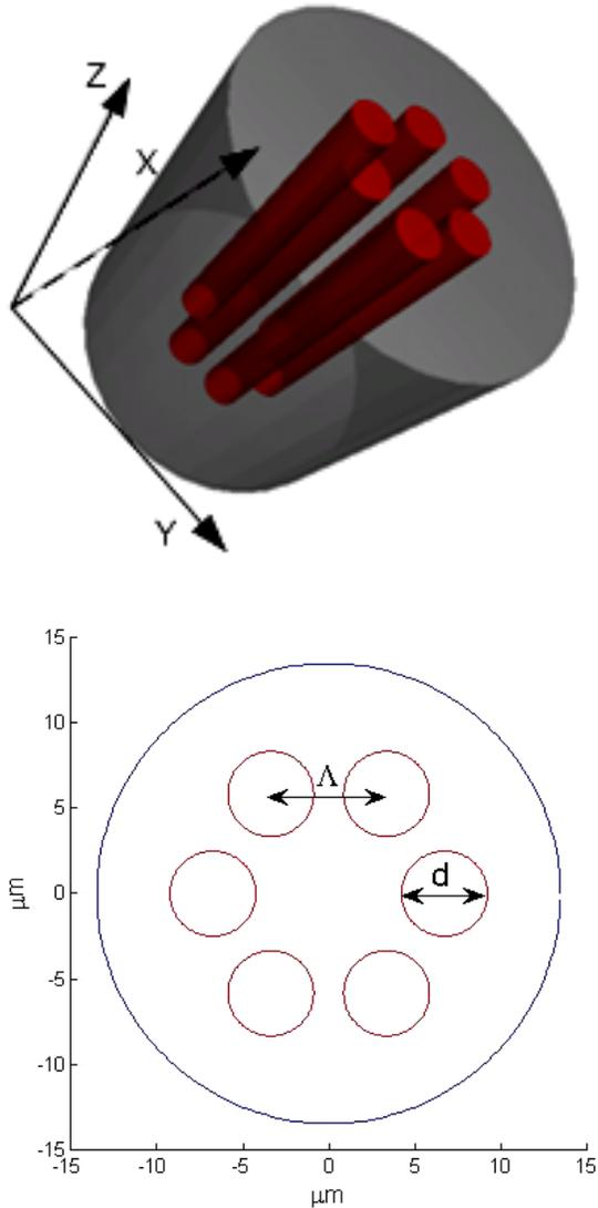
Fig.1: Permittivity distribution of the one-ring of air holes PCF structure.
