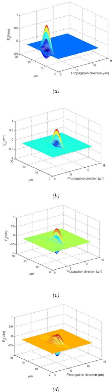
Fig.2: Propagating pulse (a) shows the pulse entering the problem space after 9 fs, (b) shows the pulse reaching the midpoint of the space after 38 fs, (c) shows the pulse which has propagated for 15  $\mu\text{m}$  after 77 fs and (d) shows the pulse which has propagated 30.7  $\mu\text{m}$  after 154 fs.
