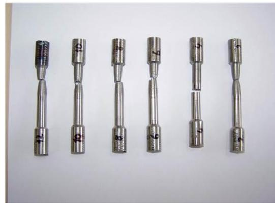
Fig. 7. Optical macro-photo of tensile test results of friction-welded joints.
