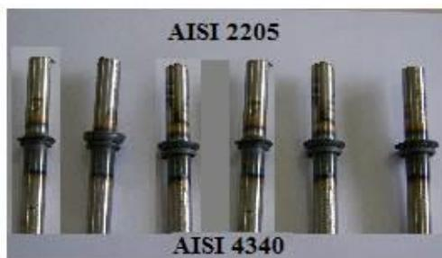
Fig. 2. Overview of friction welded AISI 4340-AISI 2205 steels.
