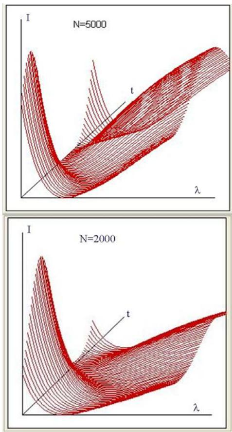
Fig. 3. Transmitted light intensity for two cells with different thicknesses ( $N$  - the number of LC layers).
