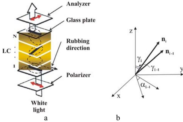
Fig. 1. a) LC cell geometry and the molecular director rotation as a result of electric field and surface interactions; b) Molecular director direction in the layers “ $i$ ” and “ $i-1$ ” and the angles used in the theoretical model.
