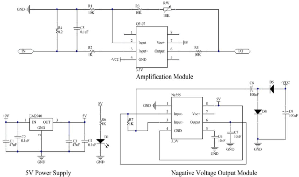
Fig. 4. Schematic diagram of sampling circuit
