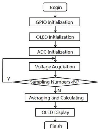
Fig. 5. Software design flow chart
