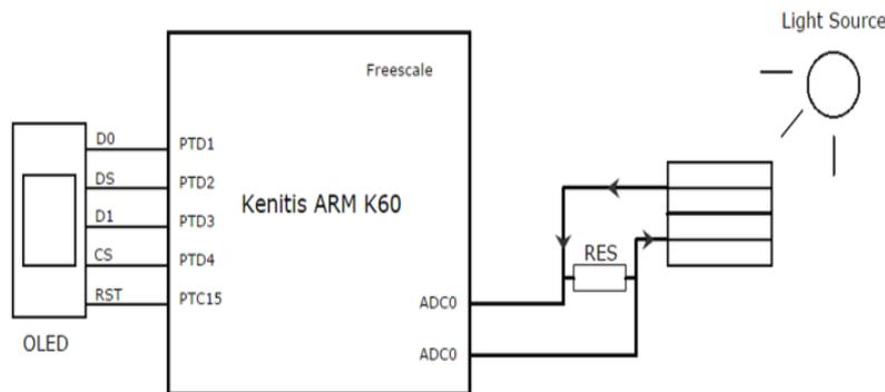
Fig. 3. Hardware block diagram of the system
