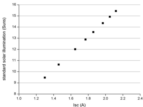
Fig. 6. The relationship between solar number and short-circuit current
