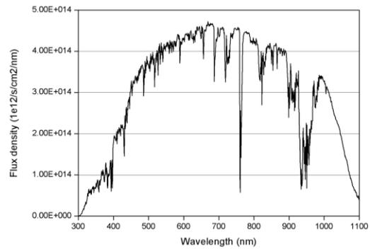
Fig. 1. Photonic flow density spectrum of sunlight (ASTM-IEC)
