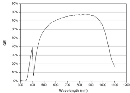
Fig. 2. QE test result of the cell
