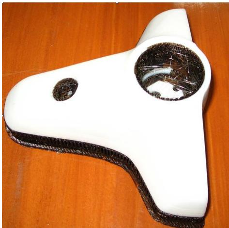
Fig. 12. The tap part formed at the rapid prototyping machine of the fused deposition modeling (FDM).
