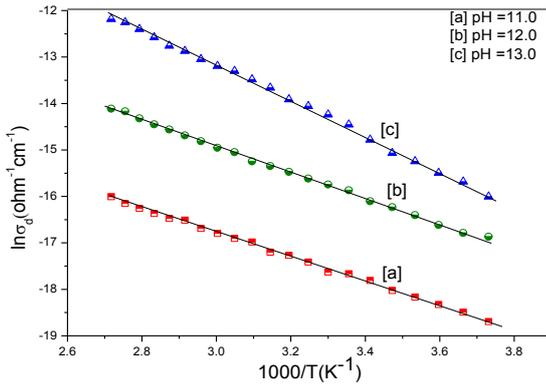
Fig. 5. Plot of (i)  $\log \sigma_d$  vs.  $(1000/T)$  of ZnSe films deposited at [a] pH = 11.0 [b] pH = 12.0 and [c] pH = 13.0.
