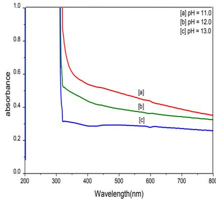
Fig. 3. Absorbance spectra of ZnSe thin films at [a] pH= 11.0 [b] pH=12.0 and [c] pH = 13.0
