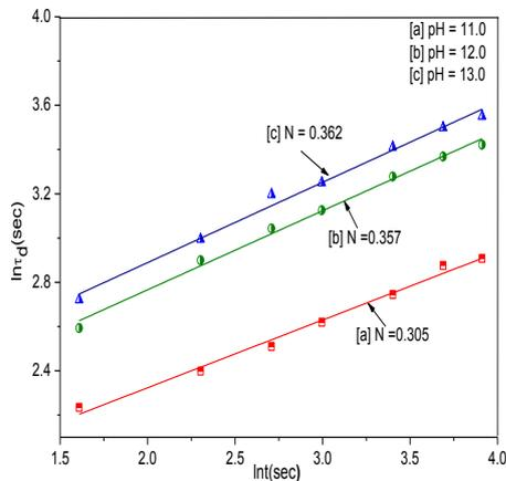
Fig. 8. Plot of  $\tau_d$  vs.  $\ln t$  for ZnSe thin films deposited at different pH [a] 11.0, [b] 12.0 and [c] 13.0.
