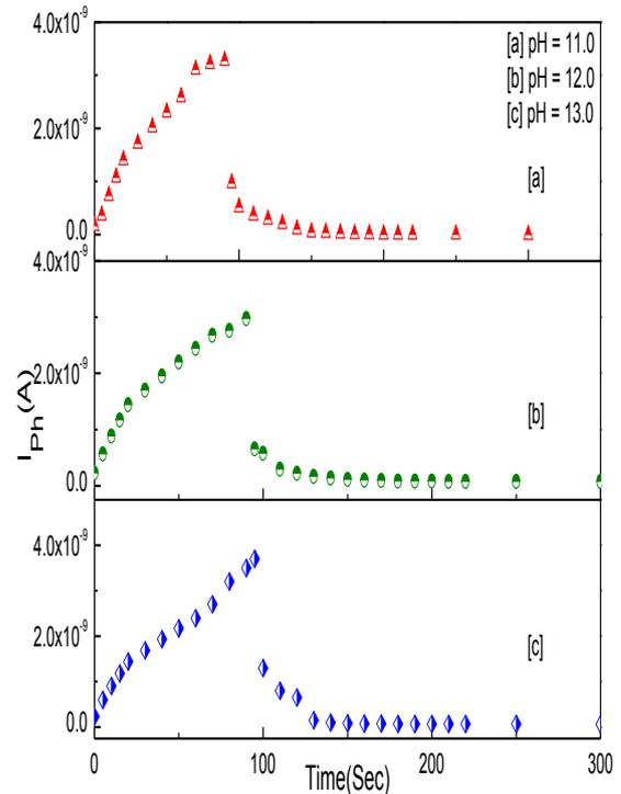
Fig. 7. The rise and decay curves of  $I_{ph}$  for ZnSe thin films at [a] pH = 11.0, [b] pH = 12.0 and [c] pH = 13.0.
