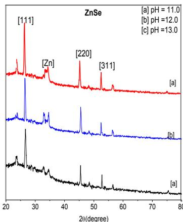
Fig. 1. XRD pattern of ZnSe thin films deposited at [a] pH=11.0 [b] pH=12.0 and [c] pH=13.0
