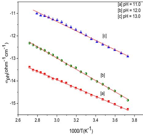
Fig. 6. Plot of  $\log \sigma_{ph}$  vs.  $(1000/T)$  of ZnSe films deposited at [a] pH = 11.0 [b] pH = 12.0 and [c] pH = 13.0.
