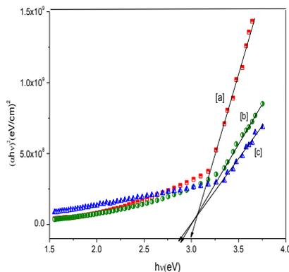
Fig. 4. The plots of  $(ahv)^2$  vs.  $hv$  for ZnSe thin films at [a] pH= 11.0 [b] pH=12.0 and [c] pH = 13.0.
