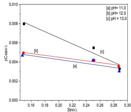
Fig. 2. Plots of  $(\beta\cos\theta)/\lambda$  vs  $(\sin\theta)/\lambda$  for ZnSe thin films at [a] pH= 11.0 [b] pH=12.0 and [c] pH = 13.0
