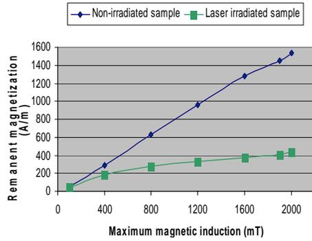
Fig. 5. Remanent magnetization vs. maximum magnetic induction.
