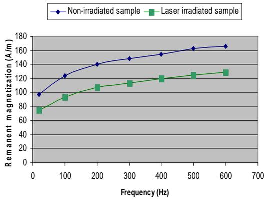
Fig. 6. Remanent magnetization vs. magnetic field frequency.
