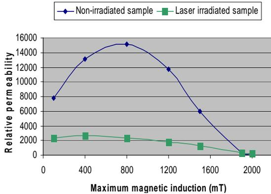
Fig. 1. Relative permeability vs. maximum magnetic induction.
