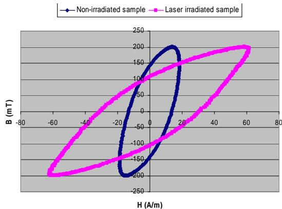
Fig. 8. Hysteresis loop ( $B_{max} = 0.2$  T,  $\nu = 200$  Hz).
