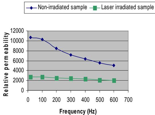
Fig. 2. Relative permeability vs. magnetic field frequency.
