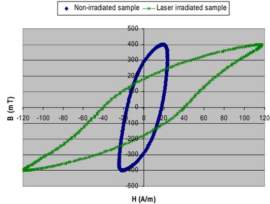
Fig. 7. Hysteresis loop ( $B_{max} = 0.4$  T,  $\nu = 100$  Hz).
