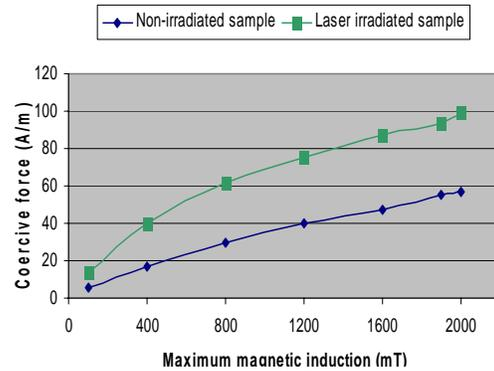
Fig. 3. Coercive force vs. maximum magnetic induction.
