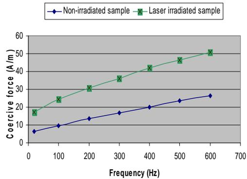
Fig. 4. Coercive force vs. magnetic field frequency.
