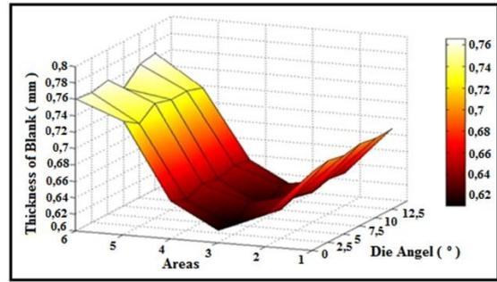
Fig. 5. Changes in thickness vs. position along sectional cut.
