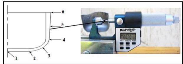
Fig. 6. Changes in thickness vs. position along sectional cut.
