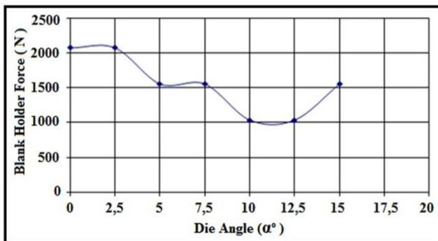
Fig. 8. Influence of  $\alpha$  angle on drawing ratio and blank holder force.
