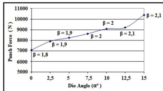
Fig. 7. Influence on punch forces of  $\alpha$  angle at the optimal deep drawing.
