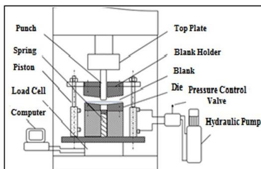
Fig. 1. The experimental setup used for deep drawing.
