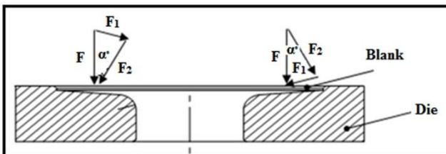
Fig. 9. Radial and axial forces over the blank.
