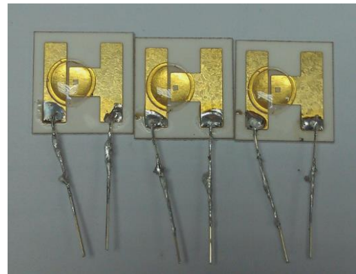
Fig. 4. LED devices interconnected by 80Au20Sn.
