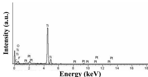
Fig. 3. EDX spectrum of sample C2.
