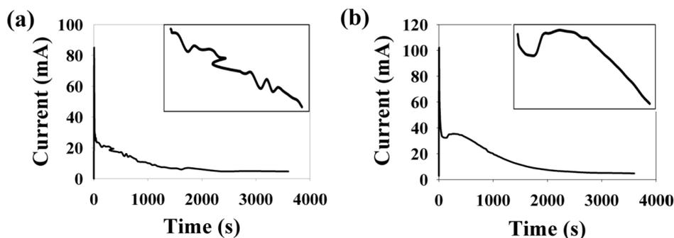
Fig. 4. Current transient profile for sample (a) A1 and (b) B1. Insets are magnification of current from 50s to 750s.
