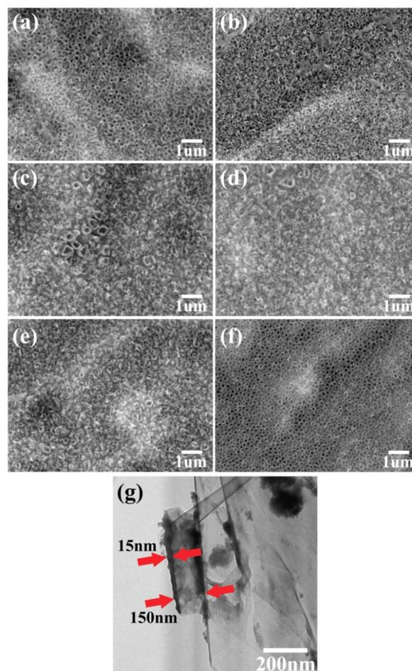
Fig. 2. SEM images with 10k magnification, top view of  $\text{TiO}_2$  nanotube samples (a) A1, (b) A2, (c) B1, (d) B2, (e) C1, (f) C2 formed under different environment and (g) EF-TEM images of C2.
