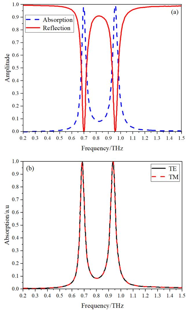
Fig. 2. Terahertz spectrum of sensor without sample in microfluidic channel. (a) absorption and reflection spectrum; (b) absorption spectrum of sensors under polarized electromagnetic waves of TE and TM
