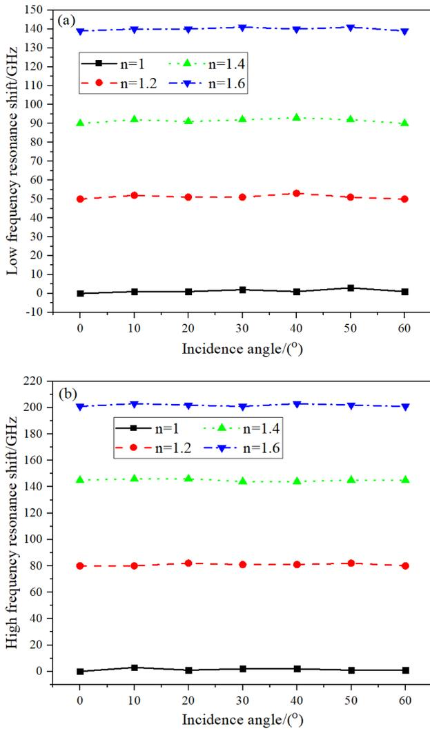
Fig. 4. Variation of absorptivity and frequency shift of sensor with incident angle. (a) low frequency resonance; (b) high frequency resonance (color online)
