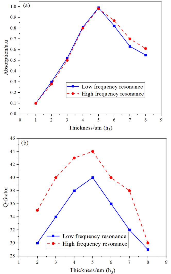
Fig. 5. Variation of absorptivity and Q value of low-frequency and high-frequency resonant points of sensors with the height of microfluidic channel (color online)
