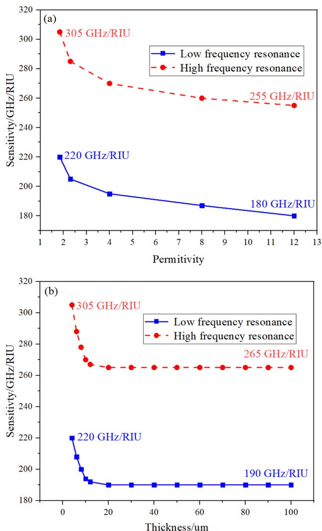
Fig. 6. Effect of dielectric constant and thickness of dielectric layer on the sensitivity of high and low absorption peaks of the sensor (color online)
