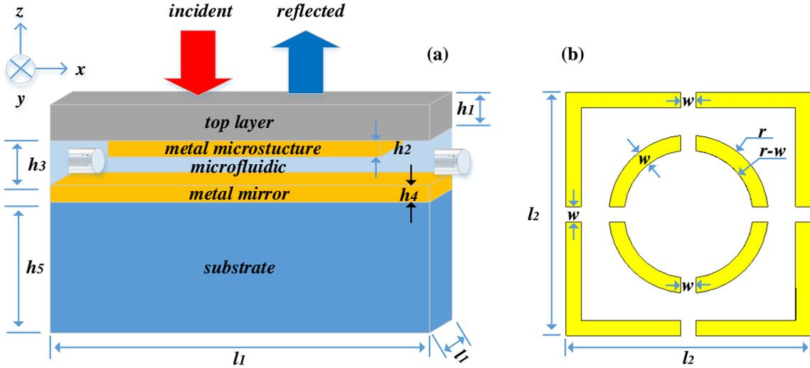
Fig. 1. Schematic diagram of unit structure of terahertz sensor. (a) side view of unit structure; (b) metal microstructure unit of sensor (color online)
