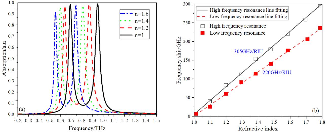
Fig. 3. Refractive index detection characteristics of sensor. (a) absorbers for samples with different refractive index; (b) linear fitting and simulation of frequency shift of high and low resonant (color online)
