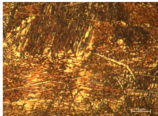
Fig. 8. Magnified OM micrograph of 473K-tempered specimen C2, revealing a series of morphologic characteristics of bainite.
