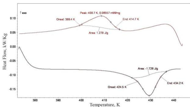
Fig. 2. DSC thermograph of normalized specimen C0, during a cooling-heating cycle, between 373 and 473 K, with  $1.67 \times 10^{-1} \text{ K} \cdot \text{sec}^{-1}$ .
