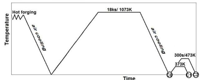
Fig. 1 Thermomechanical processing diagram of Cu-15Zn-6Al SMA. C0-normalized specimen; C1-specimen tempered at 373K; C2-specimen tempered at 473K.
