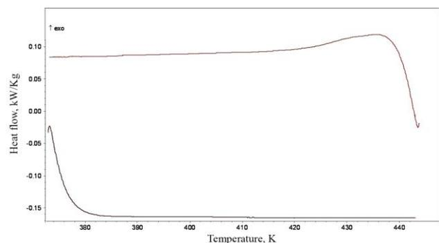
Fig. 4. DSC thermograph of tempered specimen C2, during a cooling-heating between 373 and 473 K, with  $1.67 \times 10^{-1} \text{ K} \cdot \text{sec}^{-1}$ .
