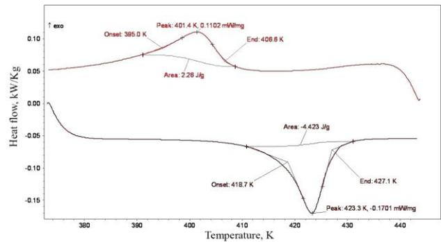
Fig. 3. DSC thermograph of tempered specimen C1 during a cooling-heating cycle, between 373 and 473 K, with  $1.67 \times 10^{-1} \text{ K} \cdot \text{sec}^{-1}$ .
