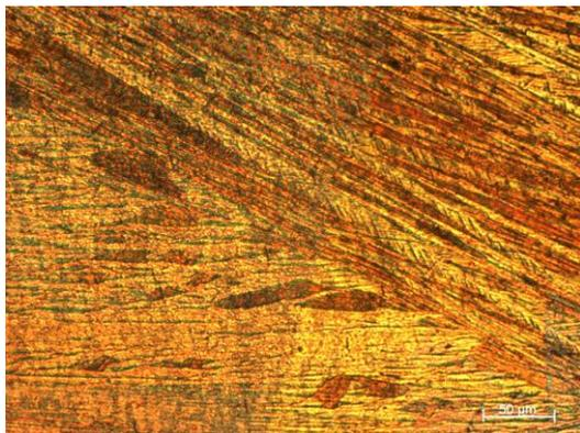
Fig. 6. OM micrograph of 373 K-tempered specimens C1, revealing long parallel martensite plates.
