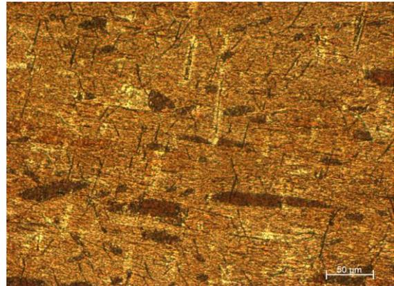
Fig. 7. OM micrograph of 473K-tempered specimen C2, revealing the absence of martensite plates.
