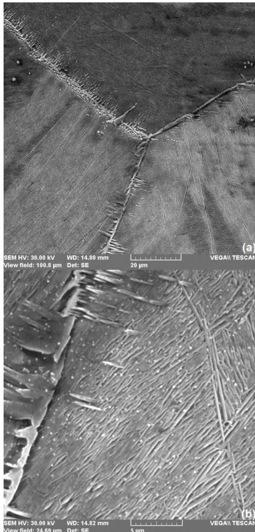
Fig. 9. SEM micrograph of 473 K-tempered specimens C2: (a) intersection area between three crystalline grains; (b) detail of the lower grain boundary, revealing a matrix with characteristic morphologic features of bainite.
