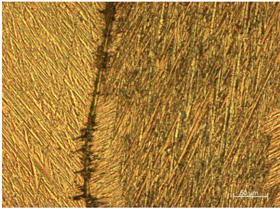
Fig. 5. OM micrograph of normalized specimen C0, revealing short martensite plates with diamond structure.
