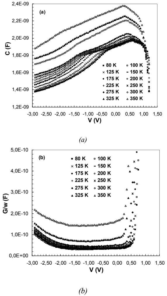
Fig.1. Capacitance-voltage (C-V) and conductance-voltage (G/w-V) characteristics of Au/SiO<sub>2</sub>/n-GaAs structure for different temperatures.
