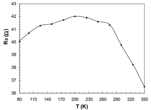
Fig. 3. Series resistance-temperature ( $R_s-T$ ) characteristics of Au/SiO<sub>2</sub>/n-GaAs structure.
