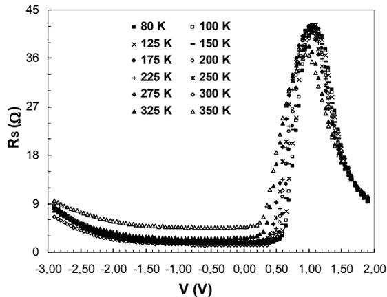
Fig. 2. Series resistance-voltage ( $R_s-V$ ) characteristics of Au/SiO<sub>2</sub>/n-GaAs structure for different temperatures.
