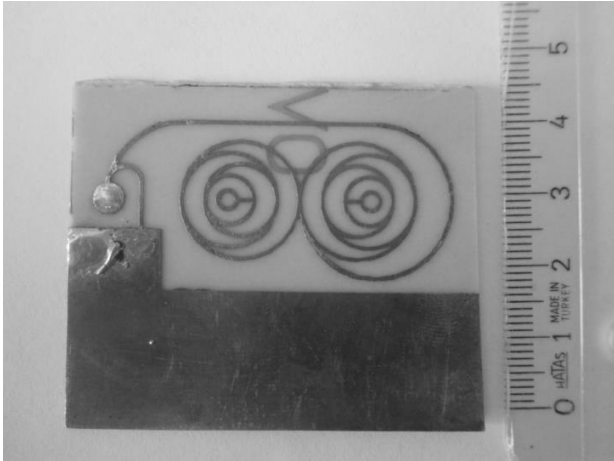
Fig. 1. Designed antenna layout on PCB.
