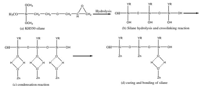
Fig. 5. Mechanism of formation of chromium-free passivation solution
