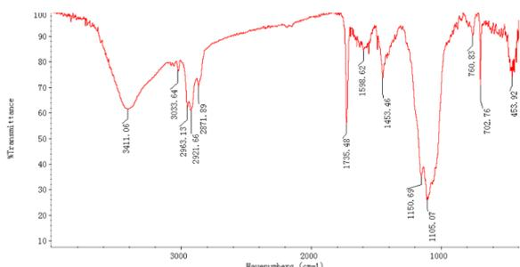
Fig. 4. IR spectrum analysis of the film
