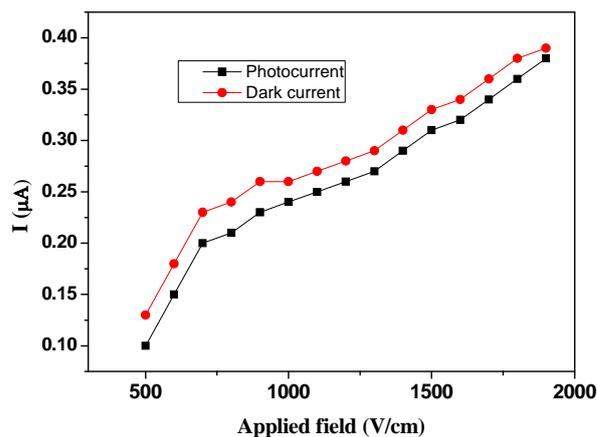
Fig. 4. Dark current and photocurrent as a function of applied field.
