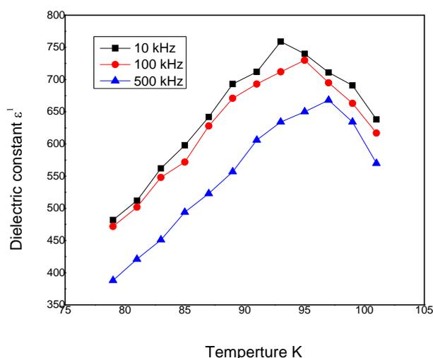
Fig. 2. Plot of dielectric constant  $\epsilon'$  against temperature at different frequencies.
