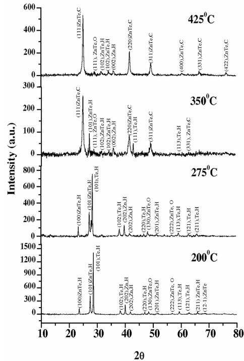
Fig. 1. XRD spectra of stacked Te and Zn layer for difference annealing temperature.
