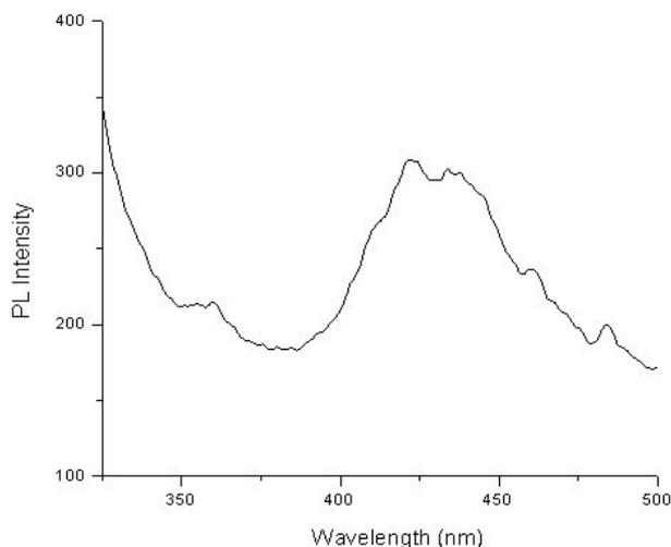
Fig. 4. Typical room-temperature photoluminescence (PL) spectrum of as-grown ZnO nanoparticles obtained by the reaction of zinc metal powder with water at 200 °C for 24h.
