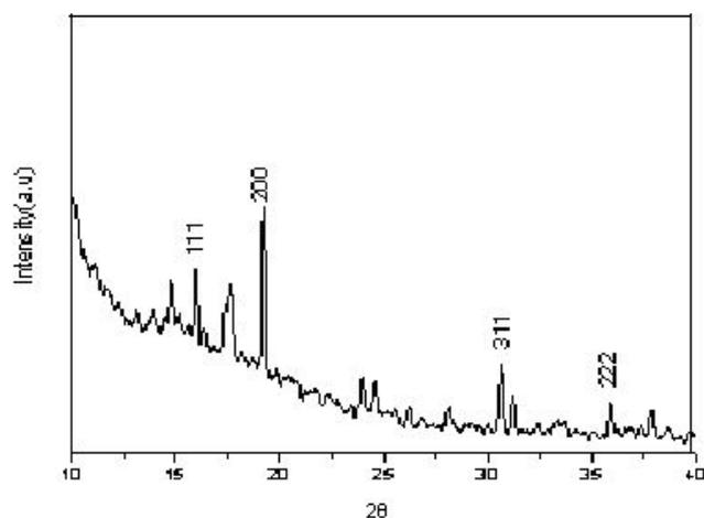
Fig. 1. Typical XRD pattern of as-grown ZnO nanoparticles obtained by the reaction of zinc metal powder with water at 200 °C for 24h.
