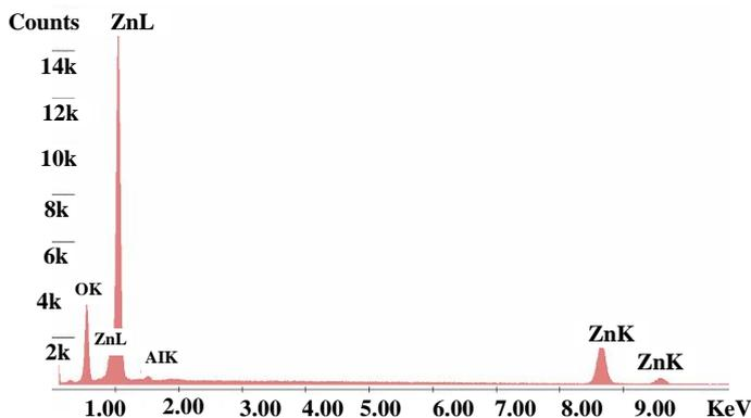
Fig. 3. Typical EDX spectrum of the as-grown ZnO nanoparticles obtained by the reaction of zinc metal powder with water at 200 °C for 24h.
