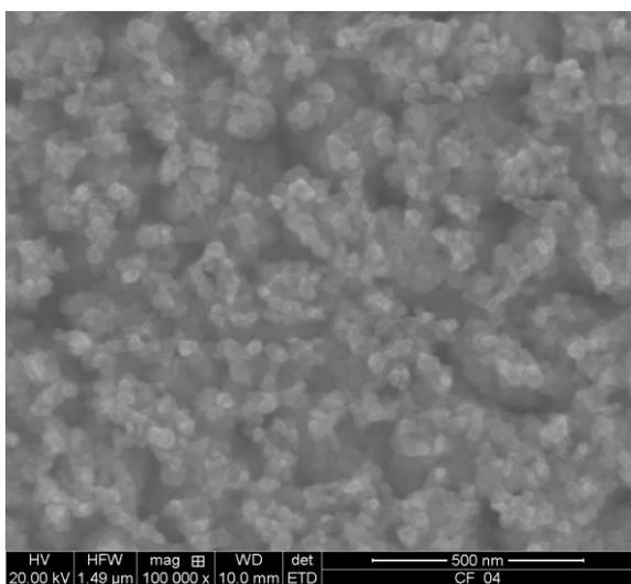
Fig. 4. SEM image of a copper nanofilm after heat treatment at the reaction temperature under vacuum condition.
