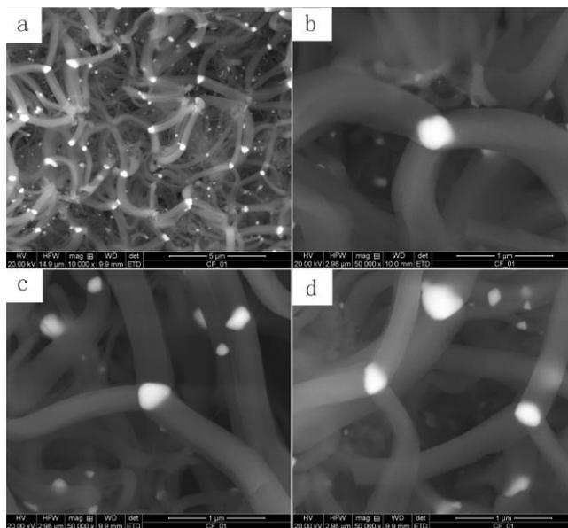
Fig. 3. SEM images of carbon nanofibers obtained on a silicon substrate. (a) Y-shaped carbon nanofibers with a diameter of circa 300 nm, copper catalyst nanoparticles with different shapes: (b) square, (c) triangular and (d) polygonal.
