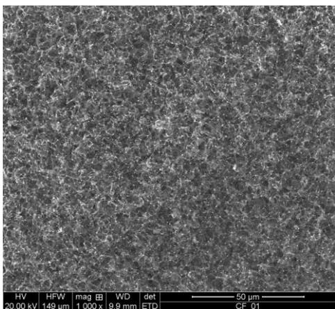
Fig. 2. SEM image of a carbon nanofiber film formed on silicon substrate.
