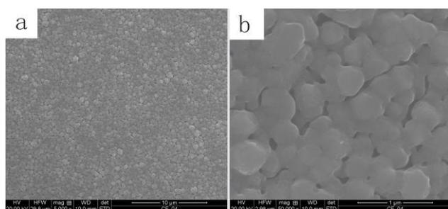
Fig. 1. SEM images of a copper nanofilms formed on silicon wafers: (a) low magnification and (b) high magnification.
