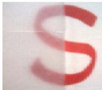
Fig. 1. Highly transparent conductive pyrrole coated NR powder /PVP composite film.
