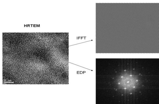
Fig. 4. HRTEM image of the nanorod with IFFT and hexagonal diffraction pattern (DP).
