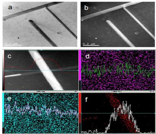
Fig. 2. (a) is transmission bright field and (b) is dark field images of plane section view of the nanorods on Si substrate. (c) Shows that oxygen is everywhere on the surface and (e) indicates the Si mapping. (f) Shows that Fe exists only at wire position.
