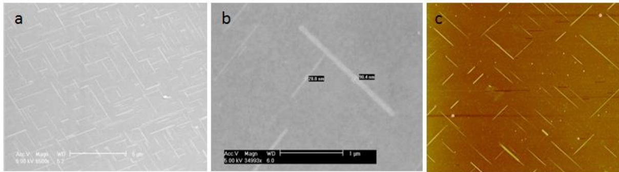
Fig. 1. (a) is SEM image of the FeO nanorods grown at Si (100), (b) is high resolution FESEM image and (c) AFM flatten image of FeO nanorods on Si surface.
