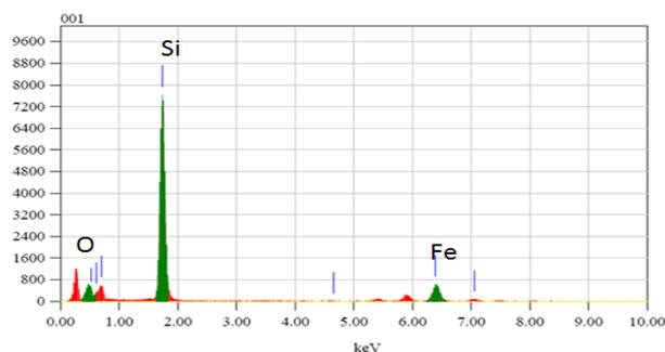
Fig. 3. EDX spectra at the nanorod position.
