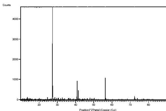
Fig. 1. powder XRD patterns of CTB crystals.
