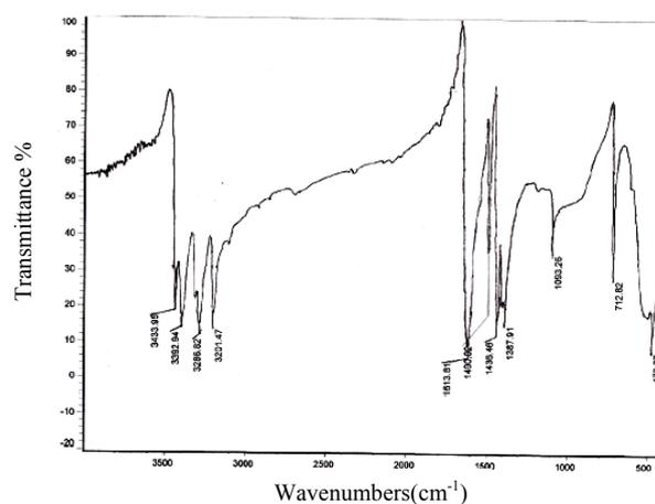
Fig. 2. FT IR Spectrum of CTB crystals.
