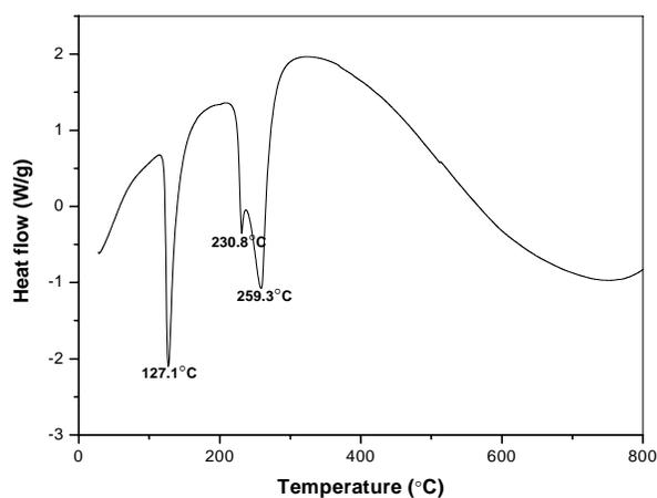
Fig. 4b. DSC curve of LPTC.
