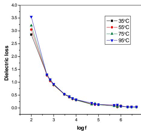
Fig. 5b. Variation of dielectric loss as a function of frequency.
