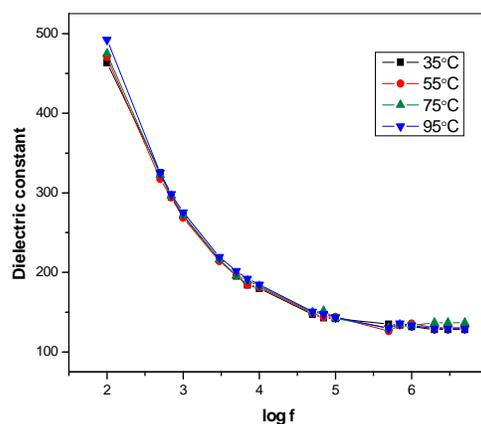
Fig. 5a. Variation of dielectric constant as a function of frequency.
