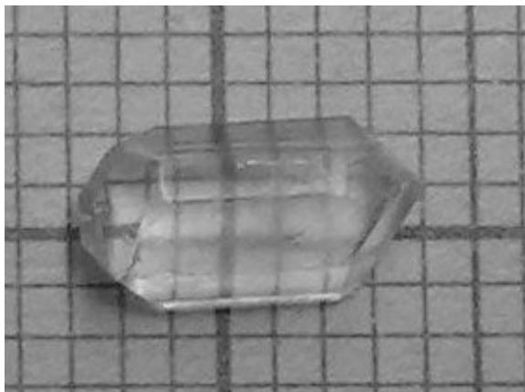
Fig. 1. As grown LPTC single crystal from aqueous solution pH of 2.0.
