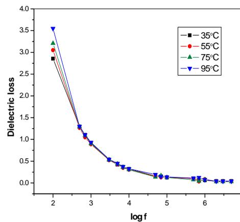
Fig. 5b. Variation of dielectric loss as a function of frequency.
