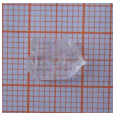
Fig. 1. As grown crystal of LPBN.
