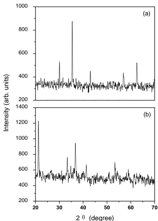
Fig. 5. XRD patterns of Fe<sub>3</sub>O<sub>4</sub> nanoparticles prepared at (a) high pH and (b) low pH.
