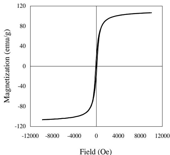
Fig. 3. Magnetic hysteresis loop of Fe<sub>3</sub>O<sub>4</sub> nanoparticles.
