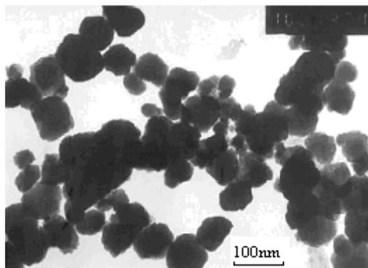
Fig. 7. TEM image of Fe<sub>3</sub>O<sub>4</sub> nanoparticles obtained at higher crystallization temperature.
