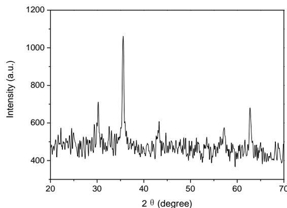
Fig. 2. XRD pattern of Fe<sub>3</sub>O<sub>4</sub> nanoparticles.
