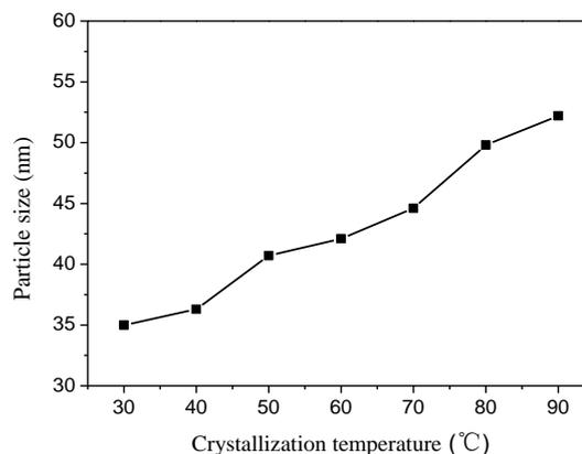
Fig. 6. Change of particle size with crystallization temperature.
