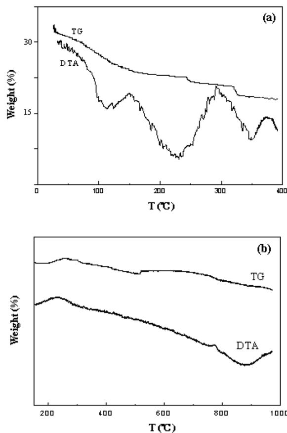
Fig. 4. TG-DTA curves during (a) dehydration process and (b) oxidation process of Fe<sub>3</sub>O<sub>4</sub> nanoparticles.
