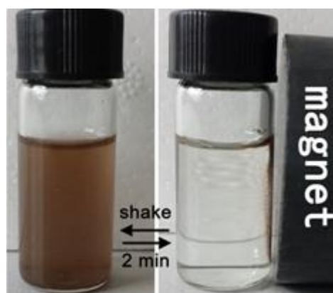
Fig. 5. Magnetic nanoparticles \text{Fe}_3\text{O}_4@/\text{SiO}_2 absorbed by magnets
