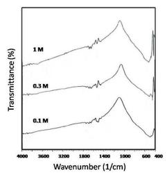
Fig. 4. FTIR spectra for: (a) 0.1 M, (b) 0.3 M, and (c) 1 M TiO<sub>2</sub> nanopowders
