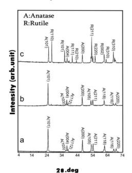
Fig. 1. The XRD pattern of (a) 0.1 M, (b) 0.3 M and (c) 1 M TiO<sub>2</sub> nanopowders
