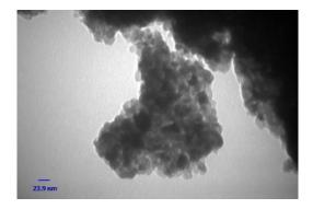
Fig. 2. Representative TEM image of TiO<sub>2</sub> nanoparticles from 0.1 M solution
