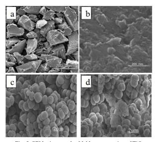
Fig. 3. SEM micrograph of 1 M concentration of TiO<sub>2</sub> nanopowders at different magnifications (a and b) and the micrograph of S. aureus (PTCC 1189) before (c) and after being damaged by TiO<sub>2</sub> nanopowders (d)
