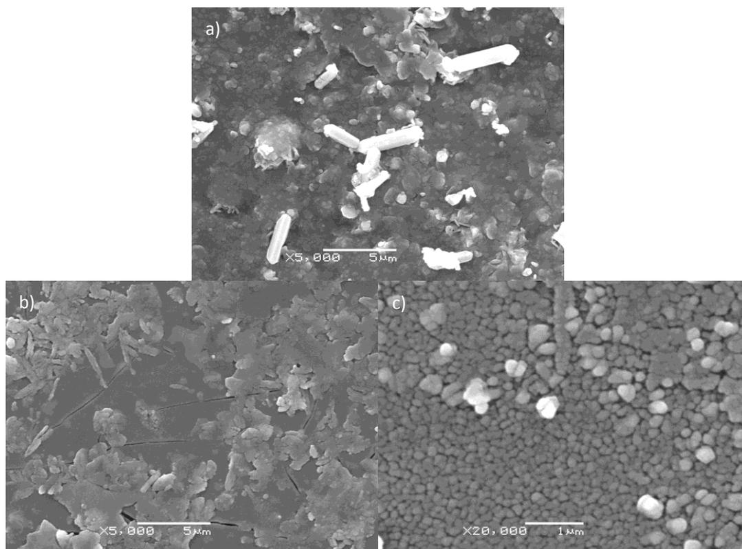
Fig. 4. SEM images of SnSe<sub>2</sub> thin films synthesized on glass substrates at 180 °C; a) 10 h, reacting twice; b and c) 20 h, reacting once.
