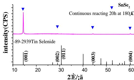
Fig. 2. The XRD pattern of SnSe<sub>2</sub> thin film synthesized on the glass substrate.
