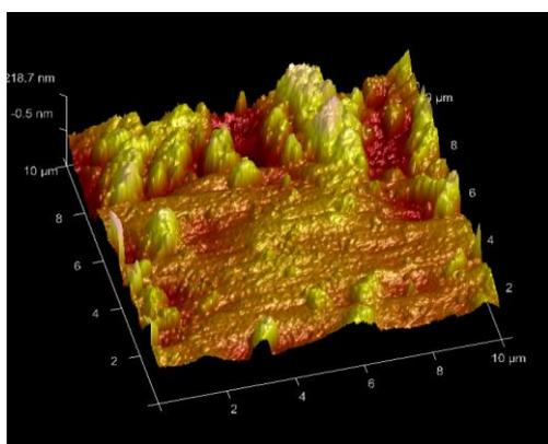
Fig. 5. The AFM image of SnSe<sub>2</sub> thin film synthesized under conditions of 180 °C+20 h on the glass substrate.
