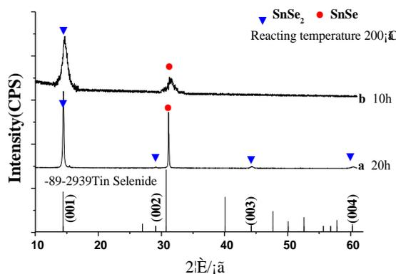
Fig. 3. XRD patterns of Sn-2Se thin films synthesized on silicon substrates Reacting time: a) 10h, b) 20h.
