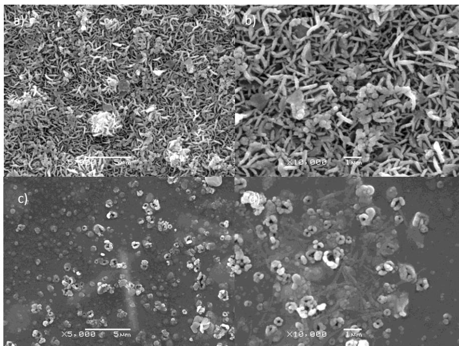
Fig. 6. The SEM images of thin film samples synthesized on silicon substrates Reacting conditions: a) and b) 200 °C+10 h, c) and d) 200 °C+20 h.
