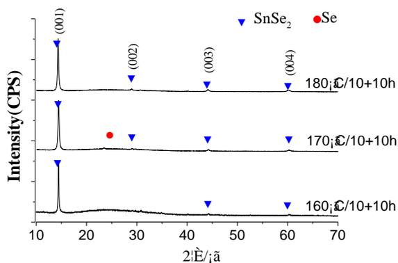
Fig. 1. XRD patterns of SnSe<sub>2</sub> thin films synthesized on the glass substrates.
