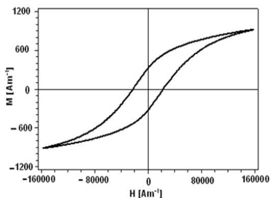
Fig. 5. Hysteresis loop of the CoFe<sub>2</sub>O<sub>4</sub> powder.
