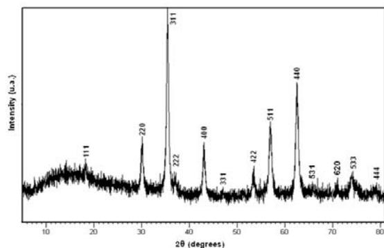
Fig. 1. XRD pattern of  $\text{CoFe}_2\text{O}_4$  powder.
