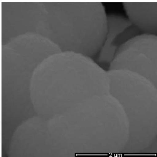
Fig. 2. SEM image of the  $\text{CoFe}_2\text{O}_4$  powder.
