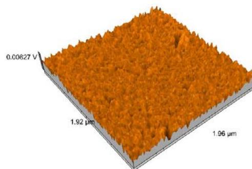
Fig. 4. AFM image: the 3D view of the cobalt spinel ferrite.
