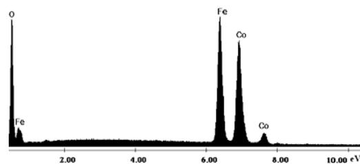
Fig. 3. The qualitative EDAX analysis for  $\text{CoFe}_2\text{O}_4$  powder.
