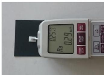
Fig. 2. Evaluation of the surface roughness, measuring surface roughness of the sintered ZrO<sub>2</sub>
