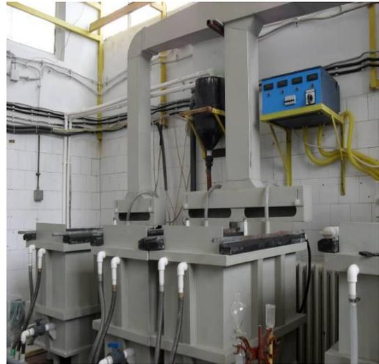
Fig. 3. Pilot plant for copper electrolytic refining.
