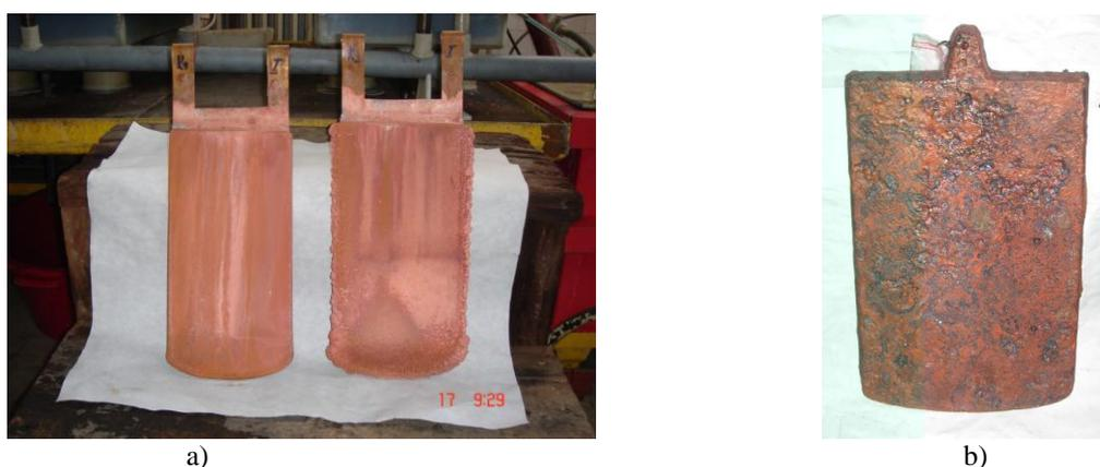
Fig. 4. a) Cathode starting sheet and cathode with deposited copper - changed shape b) Anode with changed shape.
