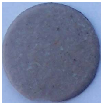
Fig. 2. The photograph of glass coating corroded in 36%HCL solution for 30 days.
