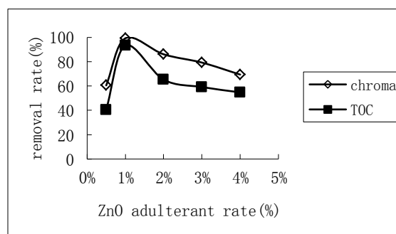
Fig. 1. The effects of ZnO adulterant proportion on the degradation activity of the photo catalyst.
