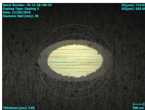
Fig. 5. AlTiN monolayer gradient coating (thickness of coating is 2.83\mu\text{m} ).
