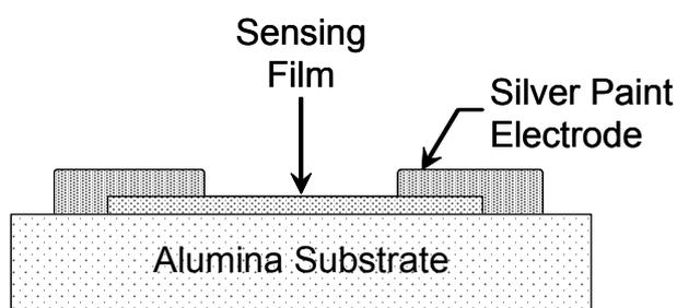
Fig. 1. Cross section of a sensor fabricated using alumina substrate.
