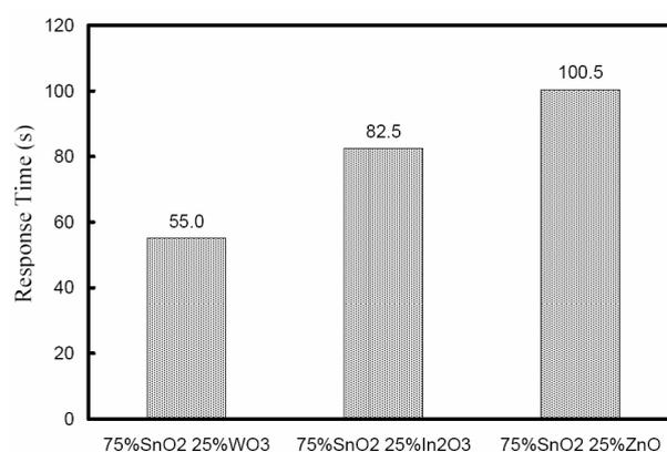
Fig. 3. Response time for binary oxides to 20 ppm isopropanol vapor.
