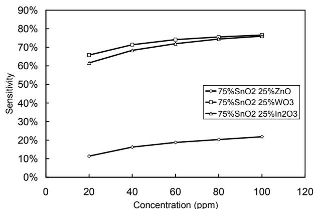
Fig. 2. Sensitivity of binary oxides of isopropanol vapors at 140 °C.
