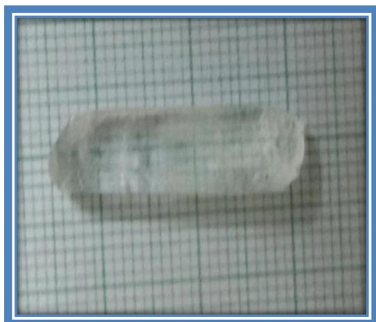
Fig. 1. Photograph of 3 wt % LC doped KDP crystal
