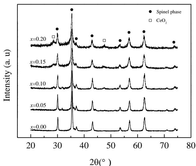
Fig. 1. X-ray diffraction patterns of  $Ni_{0.5}Zn_{0.5}Ce_xCo_{0.1}Fe_{1.9-x}O_4$  ferrite nanopowders.
