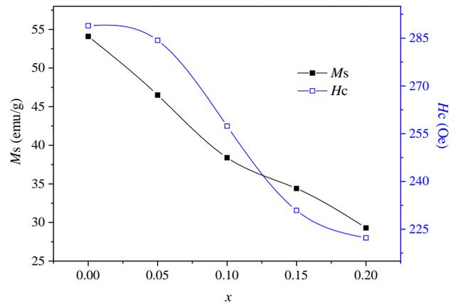
Fig. 4.  $M_s$  and  $H_c$  of  $Ni_{0.5}Zn_{0.5}Ce_xCo_{0.1}Fe_{1.9-x}O_4$  ferrite nanopowders.
