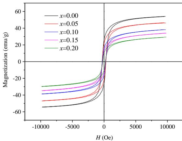
Fig. 3. Hysteresis loops of  $Ni_{0.5}Zn_{0.5}Ce_xCo_{0.1}Fe_{1.9-x}O_4$  ferrite nanopowders.
