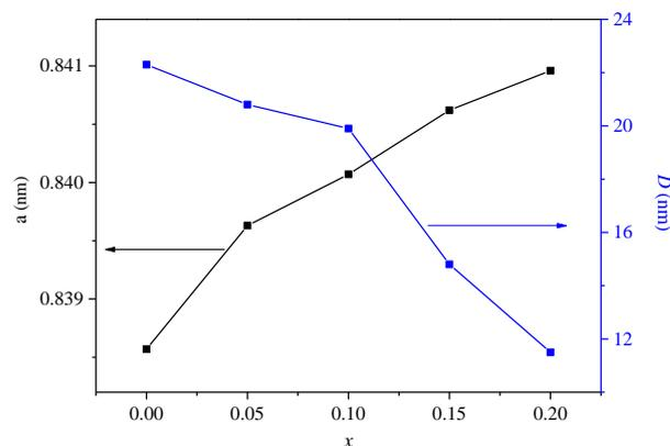
Fig. 2. Lattice parameter ( $a$ ) and average crystallite size ( $D$ ) of  $Ni_{0.5}Zn_{0.5}Ce_xCo_{0.1}Fe_{1.9-x}O_4$  ferrite nanopowders.
