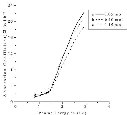
Fig. 7. Variation of absorption coefficient ( $\alpha$ ) with photon energy ( $h\nu$ ) of CuO thin films.
