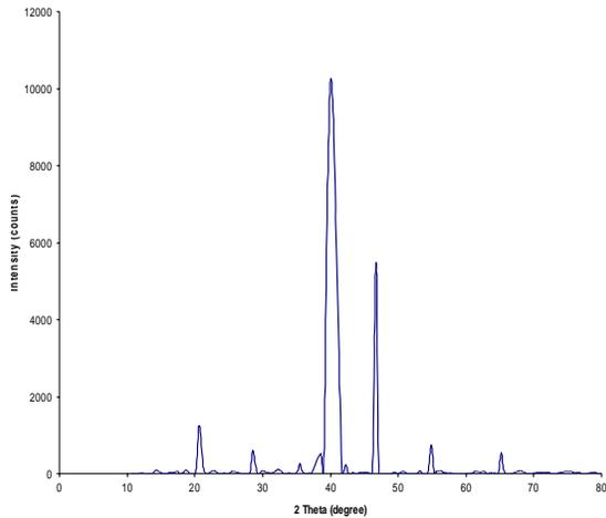
Fig. 2. Shows the X-ray diffraction pattern of CuO at 0.1 mol.
