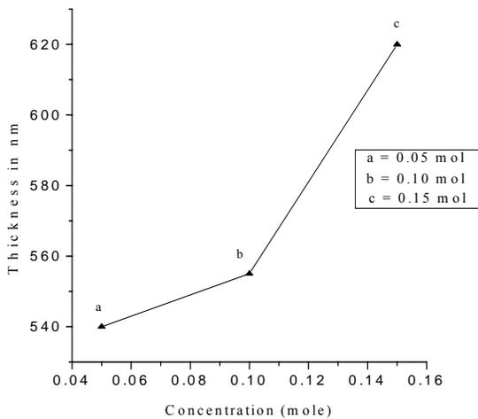
Fig. 4. Variations of film thickness Vs concentration of CuO thin film.
