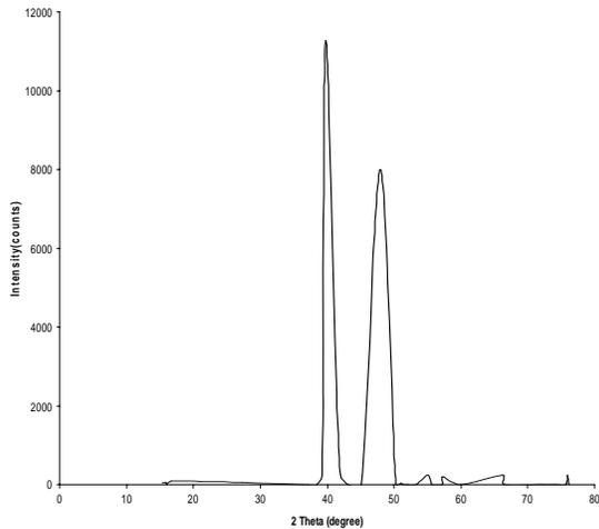
Fig. 3. Shows the X-ray diffraction pattern of CuO at 0.15 mol.
