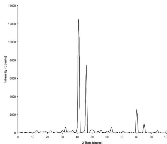
Fig. 1. Shows the X-ray diffraction pattern of CuO at 0.05 mol-concentration.
