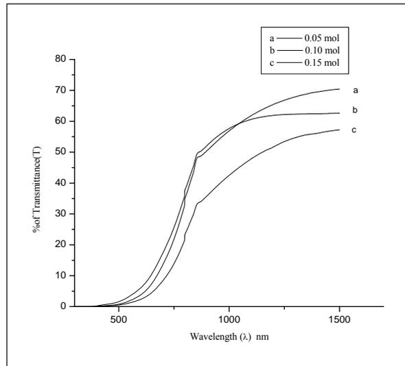
Fig. 5. Optical transmittance spectra of CuO.
