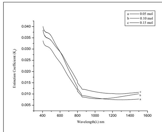
Fig. 6. Extinction coefficient CuO.
