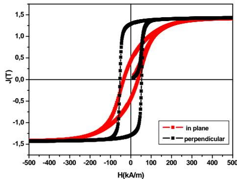
Fig. 5. Hysteresis loops of the Alnico target.
