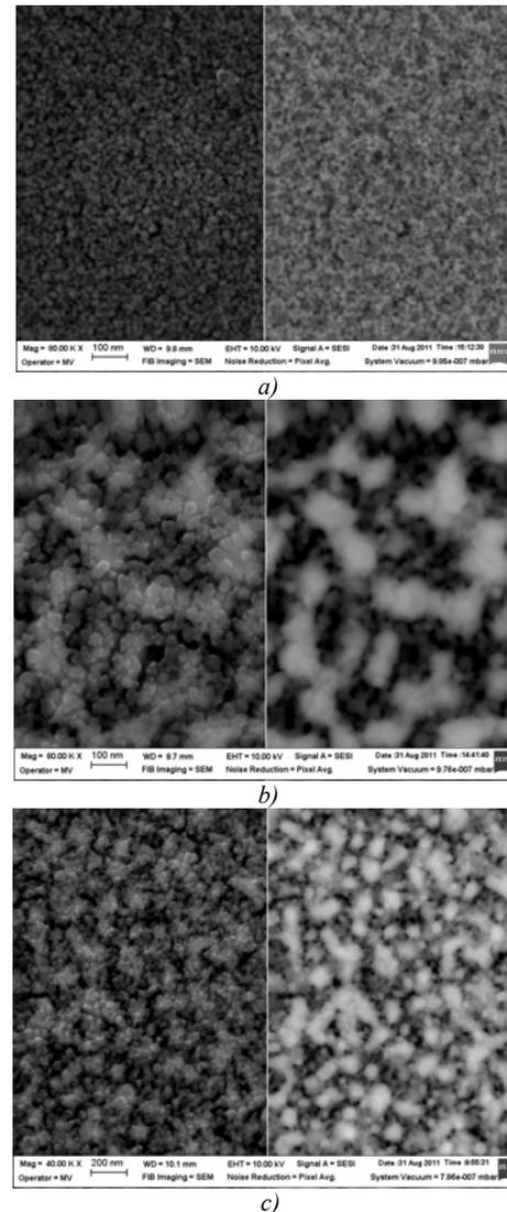
Fig. 4. SEM (left secondary electron, right backscattering electron) images: a) 50 nm thickness, b) 100 nm thickness, c) 150 nm thickness.
