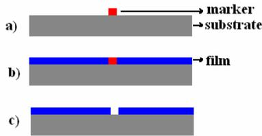
Fig. 1. A schematic representation of a) the substrate line marked before deposition process, b) the film after deposition process, c) the film after removing the marker line.
