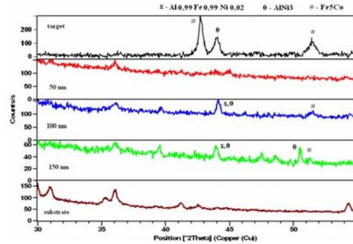
Fig. 3. XRD patterns for the target (black), the annealed films (red 50 nm thickness, blue 100 nm thickness, green 150 nm thickness) and for the ceramic substrate (brown pattern).
