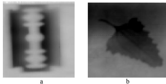
Fig. 3. Images of 2D objects: a steel razor (a), and leaf (b) hidden between layers of scattering media (see text).
