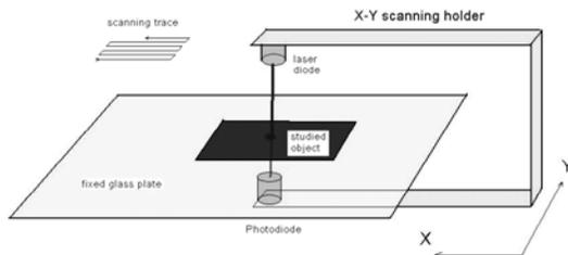
Fig. 1. Schematic drawing of 2D scanning head and unmovable object table.
