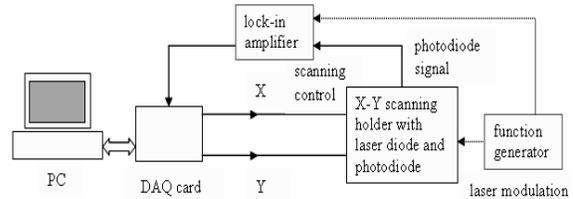
Fig. 2. Block-scheme of the experimental setup.
