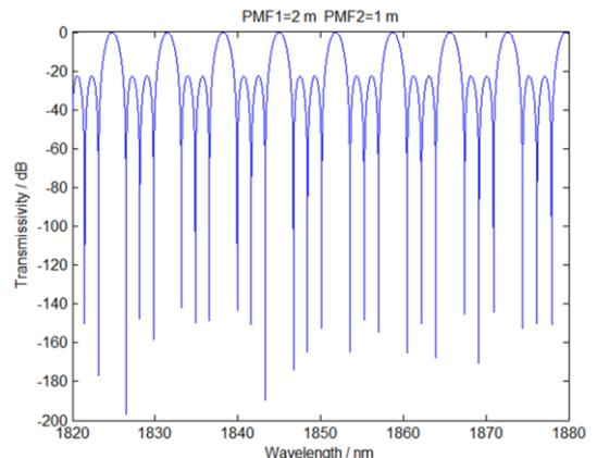
Fig. 2. Cascaded Sagnac loop simulation transmission curve
