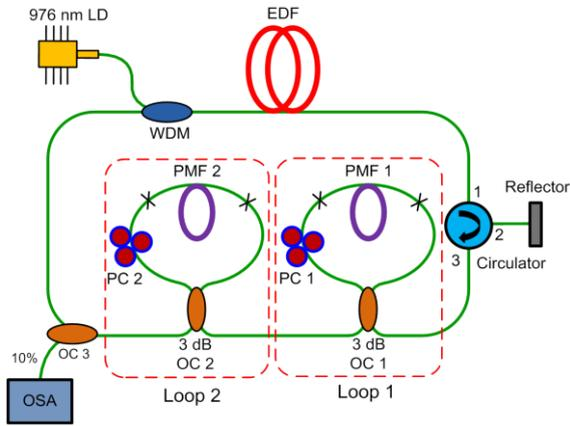
Fig. 1. Setup of the multi-wavelength laser based on double Sagnac loops
