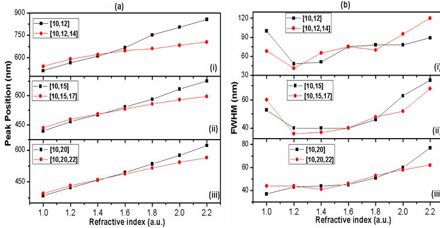
Fig. 4. Sensing responses of Ag nanoshells with different radius ratio before and after coating with 2 nm dielectric layer. (a) peak positions and (b) FWHMs vs refractive index of the surrounding environment. i) [10, 12] nm; ii) [10, 15] nm; iii) [10, 20] nm
