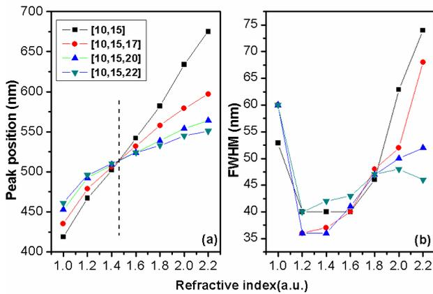
Fig. 2. Sensing responses of [10, 15] nm Ag nanoshells before and after coated with dielectric layer of different thicknesses. (a) peak positions of extinction spectra vs refractive index of the surrounding environment; (b) FWHMs vs refractive index of the surrounding environment
