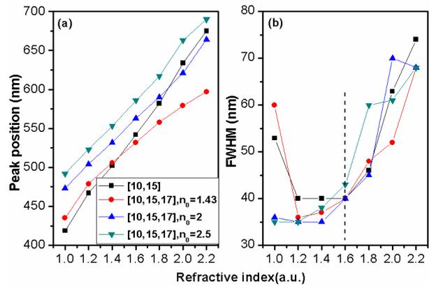
Fig. 3. Sensing responses of [10, 15] nm Ag nanoshells before and after coated with 2 nm dielectric layer of different refractive index. (a) peak positions of extinction spectra vs refractive index of the surrounding environment; (b) FWHMs vs refractive index of the surrounding environment
