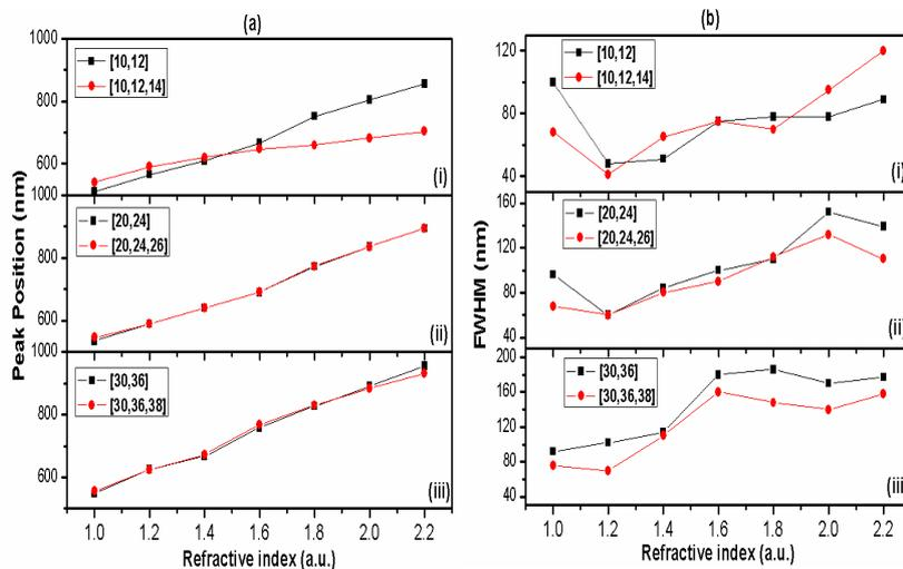
Fig. 5. Sensing responses of Ag nanoshells with different size before and after coating with 2 nm dielectric layer. (a) peak positions and (b) FWHMs vs refractive index of the surrounding environment. i) [10, 12] nm; ii) [20, 24] nm; iii) [30, 36] nm
