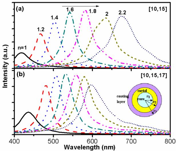
Fig. 1. LSP extinction spectra of [10, 15] nm Ag nanoshells in different dielectric environment. (a) bare Ag nanoshell; (b) after coated with 2 nm layer. Inset: Structure schematics of the dielectric-coated metal nanoshells
